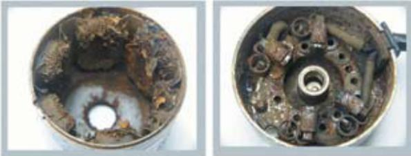
Although the outside of the starter (at bottom right) looks fine, the flywheel picked up water from the bilge and pumped it inside the starter causing the corrosion shown here.
