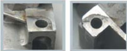
Shown here are damaged starter mounting pads. Water ingested into the engine stresses the mounting bolts beyond normal conditions. The bolts stretch and cause the starter to become loose. This could eventually lead to damage to the ring gear, starter casting and possibly the entire engine block.
